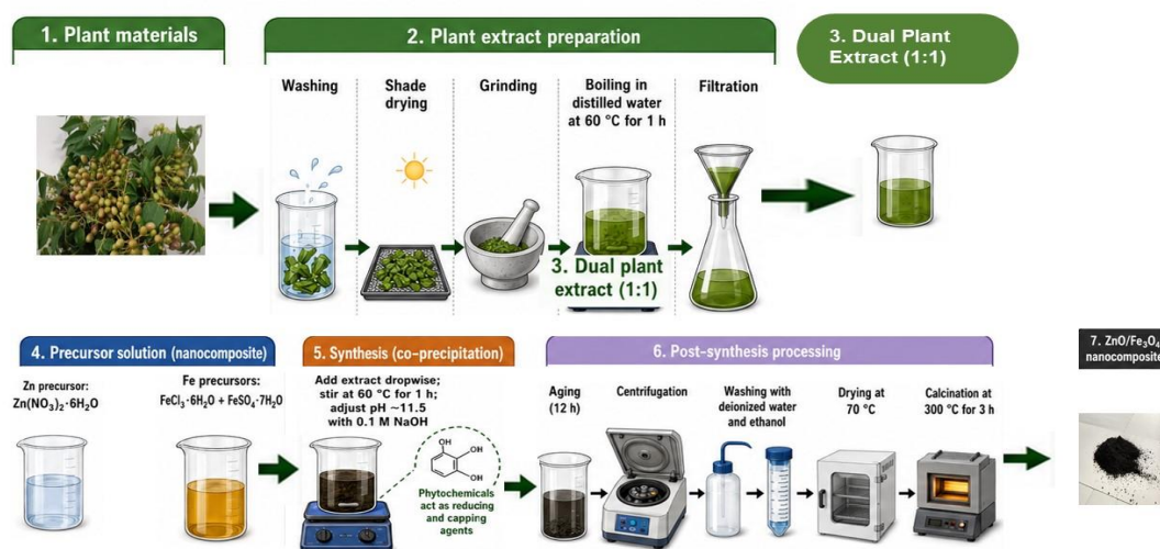
Fig (1): Schematic illustration of the green synthesis route employed for the preparation of the ZnO/Fe 3 O 4 nanocomposite using aqueous extract of fruit pods of Murraya koenigii and stems of Cissus quadrangularis in 1:1 ratio.
